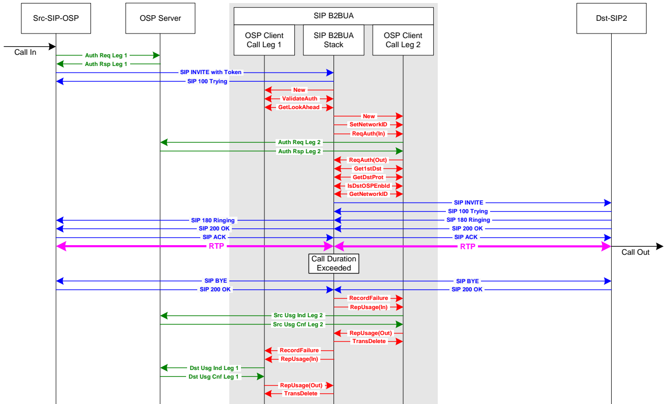
Test Case 2.3.4: OSP Source to SIP B2BUA to non-OSP Destination: Call Duration Limit Exceeded Legend: SIP Messages in Blue, OSP Toolkit Calls in Red, OSP Messages in Green
